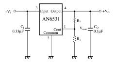
$$\begin{split} &V_{\rm O} = V_{\rm cont} \left(\frac{R_1 + R_2}{R_1}\right) \\ &(V_{\rm cont} \cong 5V, \, R_1 = 5k\Omega) \\ &C_{\rm I} \text{ is necessary when the } V_{\rm I} \text{ line is long.} \\ &C_{\rm O} \text{ improves the transient response.} \end{split}$$
