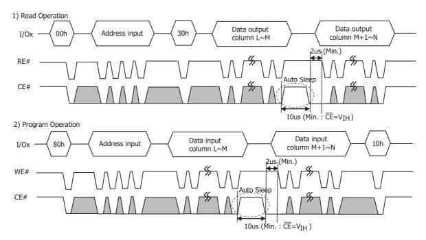
Figure 29: tCS setting when deactivating the auto sleep mode
