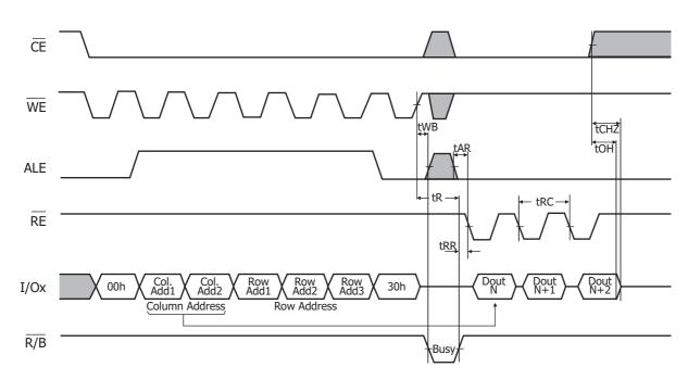
Figure 10: Read1 Operation intercepted by CE#
