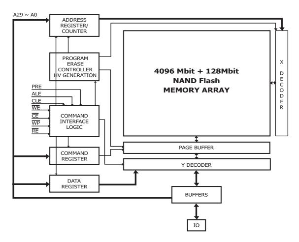
Figure 3: Block Diagram
