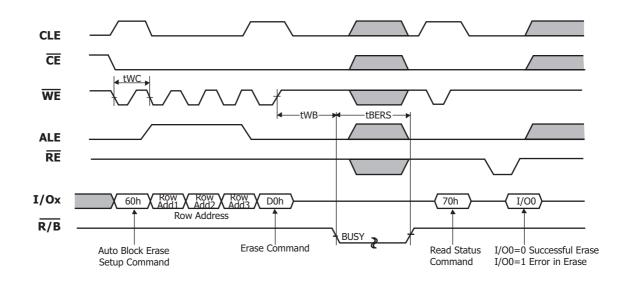
Figure 16: Block Erase Operation (Erase One Block)
