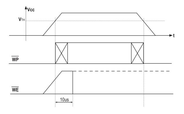
Figure 23: Power On and Data Protection Timing
