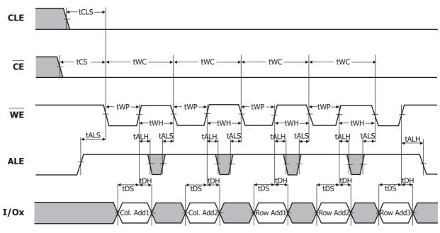
Figure 5: Address Latch Cycle
