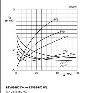
Fig.5 Temperature coefficient as a function of working current; typical values.
