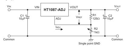
$$V_{OUT} = V_{REF} (1 + \frac{R2}{R1}) + I_{ADJ} R2$$
