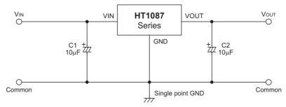
Note: C1 is required if the needed if the device is located far from filter capacitors, the recommended value is  $10\mu F$ . C2 is required for stability, the recommended value is  $10\mu F$ .
