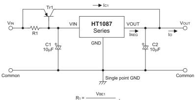
$$R_1 = \frac{V_{BE1}}{I_{REG} - \frac{I_{C1}}{(1+\beta)}}$$
