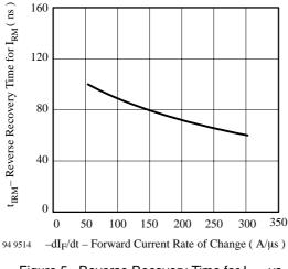
Figure 5. Reverse Recovery Time for I<sub>RM</sub> vs. Forward Current Rate of Change
