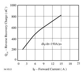
Figure 4. Reverse Recovery Charge vs. Forward Current
