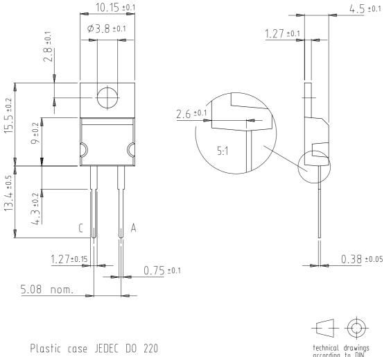
Cathode connected with metallic surface
