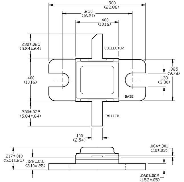
UNLESS OTHERWISE NOTED, TOLERANCES ARE INCHES ±.005\* (MILLIMETERS ±.13MM)
