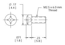
Material: Steel Plating: Zinc Thread Size: M2.5 Package Size: 200 Pieces
