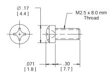
Material: Steel Plating: Zinc Thread Size: M2.5 Package Size: 200 Pieces
