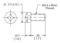
Material: Steel Plating: Zinc Thread Size: M2.6 Package Size: 200 Pieces
