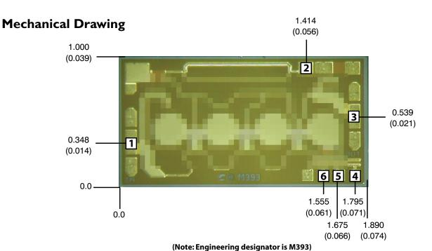
Units: millimeters (inches) Bond pad dimensions are shown to center of bond pad.
