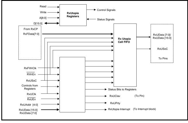
FIGURE 36. FUNCTIONAL BLOCK DIAGRAM OF THE RECEIVE UTOPIA INTERFACE BLOCK
