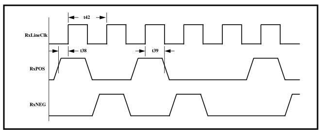
FIGURE 86. WAVEFORM/TIMING RELATIONSHIP BETWEEN RXLINECLK, RXPOS AND RXNEG - WHEN RXPOS AND RXNEG ARE TO BE SAMPLED ON THE FALLING EDGE OF RXLINECLK
