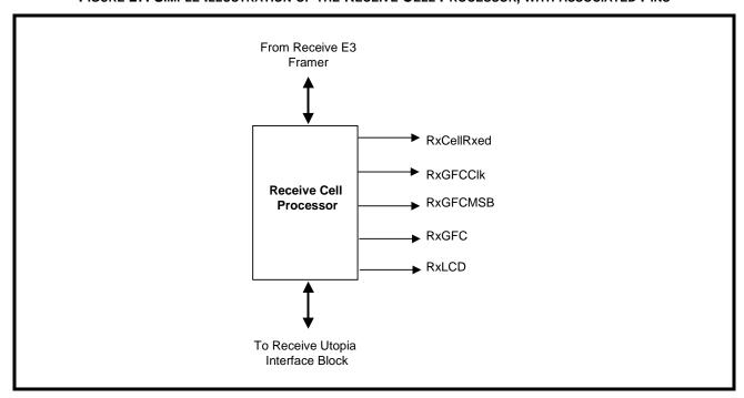
FIGURE 27. SIMPLE ILLUSTRATION OF THE RECEIVE CELL PROCESSOR, WITH ASSOCIATED PINS
