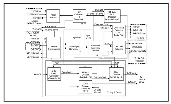
Figure 24 indicates that the PLCP Frame consists of 12 ATM Cells, 48 bytes of Overhead (OH) bytes, and 13 or 14 nibbles of "trailer" for frequency justification.
