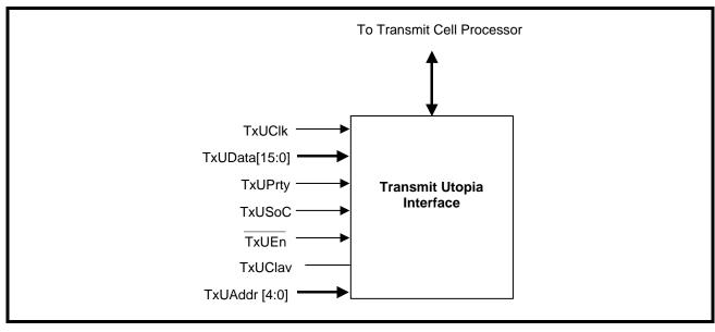
FIGURE 3. SIMPLE BLOCK DIAGRAM OF TRANSMIT UTOPIA INTERFACE
