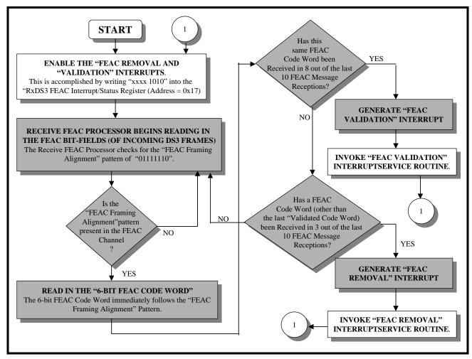
FIGURE 91. FLOW DIAGRAM DEPICTING HOW THE RECEIVE FEAC PROCESSOR FUNCTIONS
