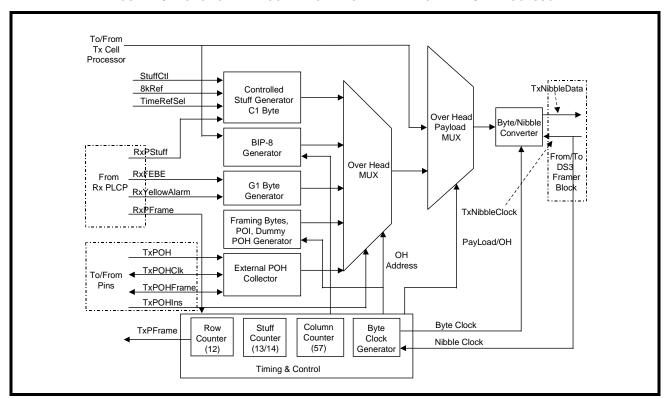
Figure 19 indicates that the Transmit PLCP Processor consists of the following functional blocks.
