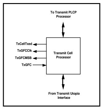
Figure 15 presents a functional block diagram of the Transmit Cell Processor.
