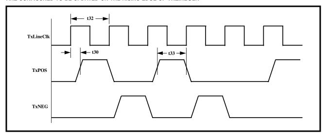
FIGURE 78. WAVEFORM/TIMING RELATIONSHIP BETWEEN TXLINECLK, TXPOS AND TXNEG - TXPOS AND TXNEG ARE CONFIGURED TO BE UPDATED ON THE FALLING EDGE OF TXLINECLK
