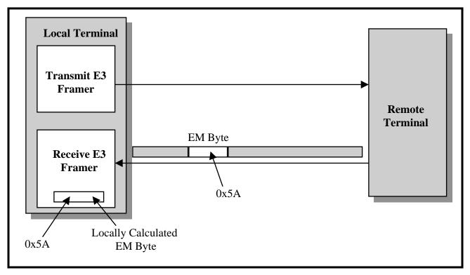
FIGURE 204. THE LOCAL RECEIVE E3 FRAMER BLOCK, TRANSMITTING AN E3 FRAME TO THE REMOTE TERMINAL WITH THE FEBE BIT WITHIN THE MA BYTE-FIELD SET TO "0"
