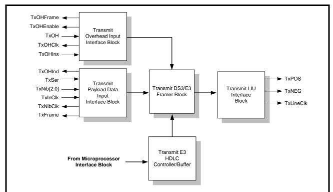
FIGURE 105. THE XRT74L73 TRANSMIT SECTION WHEN IT HAS BEEN CONFIGURED TO OPERATE IN THE E3 MODE
