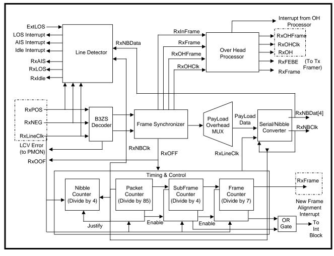
FIGURE 22. FUNCTIONAL BLOCK DIAGRAM OF RECEIVER FRAMER
