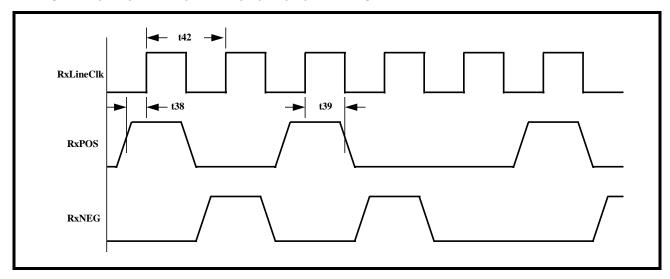
FIGURE 199. WAVEFORM/TIMING RELATIONSHIP BETWEEN RXLINECLK, RXPOS AND RXNEG - WHEN RXPOS AND RXNEG ARE TO BE SAMPLED ON THE FALLING EDGE OF RXLINECLK
