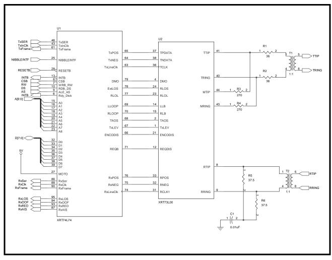
FIGURE 185. APPROACH TO INTERFACING THE XRT74L73 FRAMER IC TO THE XRT73L00 DS3/E3/STS-1 LIU
