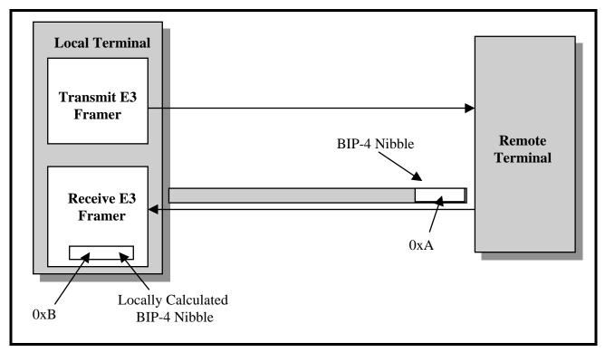
FIGURE 148. THE LOCAL RECEIVE E3 FRAMER BLOCK, TRANSMITTING AN E3 FRAME TO THE REMOTE TERMINAL WITH THE "A" BIT-FIELD SET TO "1"
