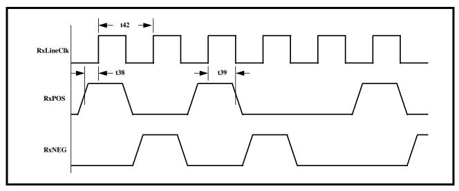
FIGURE 141. WAVEFORM/TIMING RELATIONSHIP BETWEEN RXLINECLK, RXPOS AND RXNEG - WHEN RXPOS AND RXNEG ARE TO BE SAMPLED ON THE FALLING EDGE OF RXLINECLK
