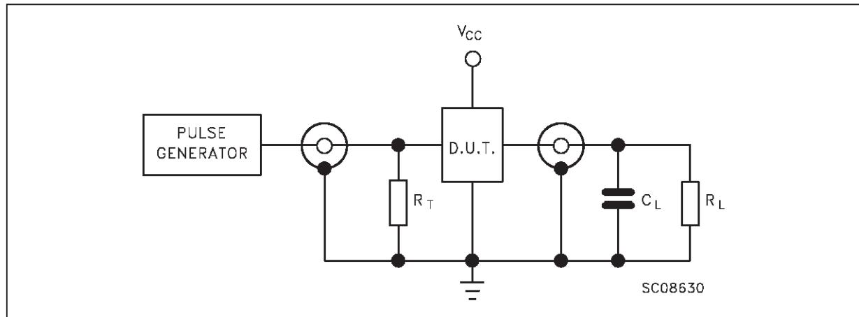
$C_L = 50 \text{ pF}$  or equivalent (includes jig and probe capacitance)
