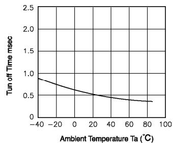
**Fig.5** LED operate vs. ambient temperature
