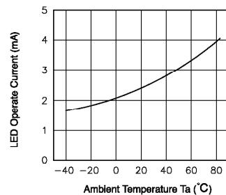
**Fig.6** LED turn off current vs. ambient
