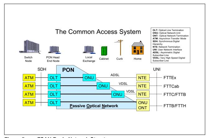
Figure 5 FSAN Basic Network Structure
