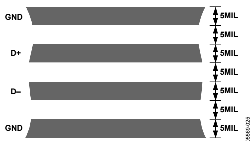
Figure 35. Typical Arrangement of Signal Tracks
