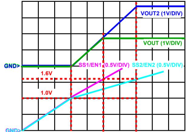
FIGURE 6. VOLTAGE TRACKING
