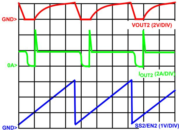
FIGURE 12. OVERCURRENT PROTECTION
