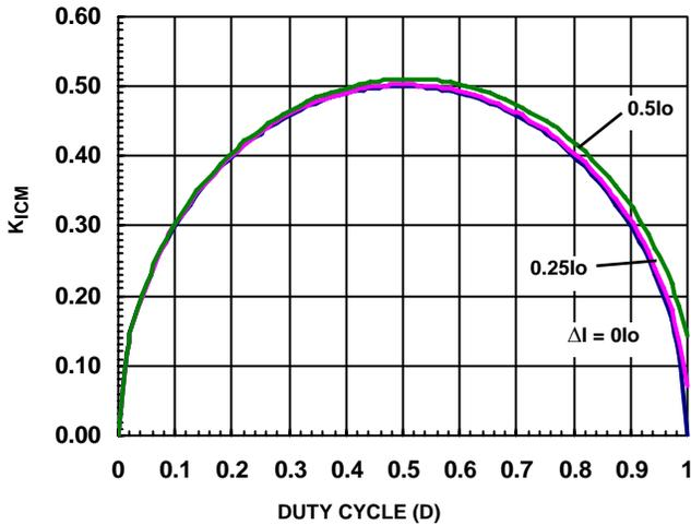
**FIGURE 11. INPUT-CAPACITOR CURRENT MULTIPLIER FOR SINGLE-PHASE BUCK CONVERTER**
