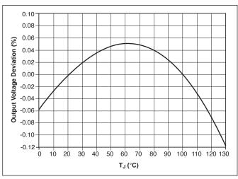
Output Voltage vs. Temperature
