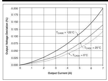
Load Regulation vs. Output Current
