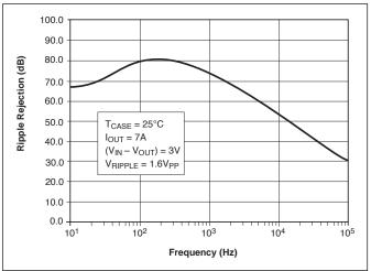
Ripple Rejection vs Frequency
