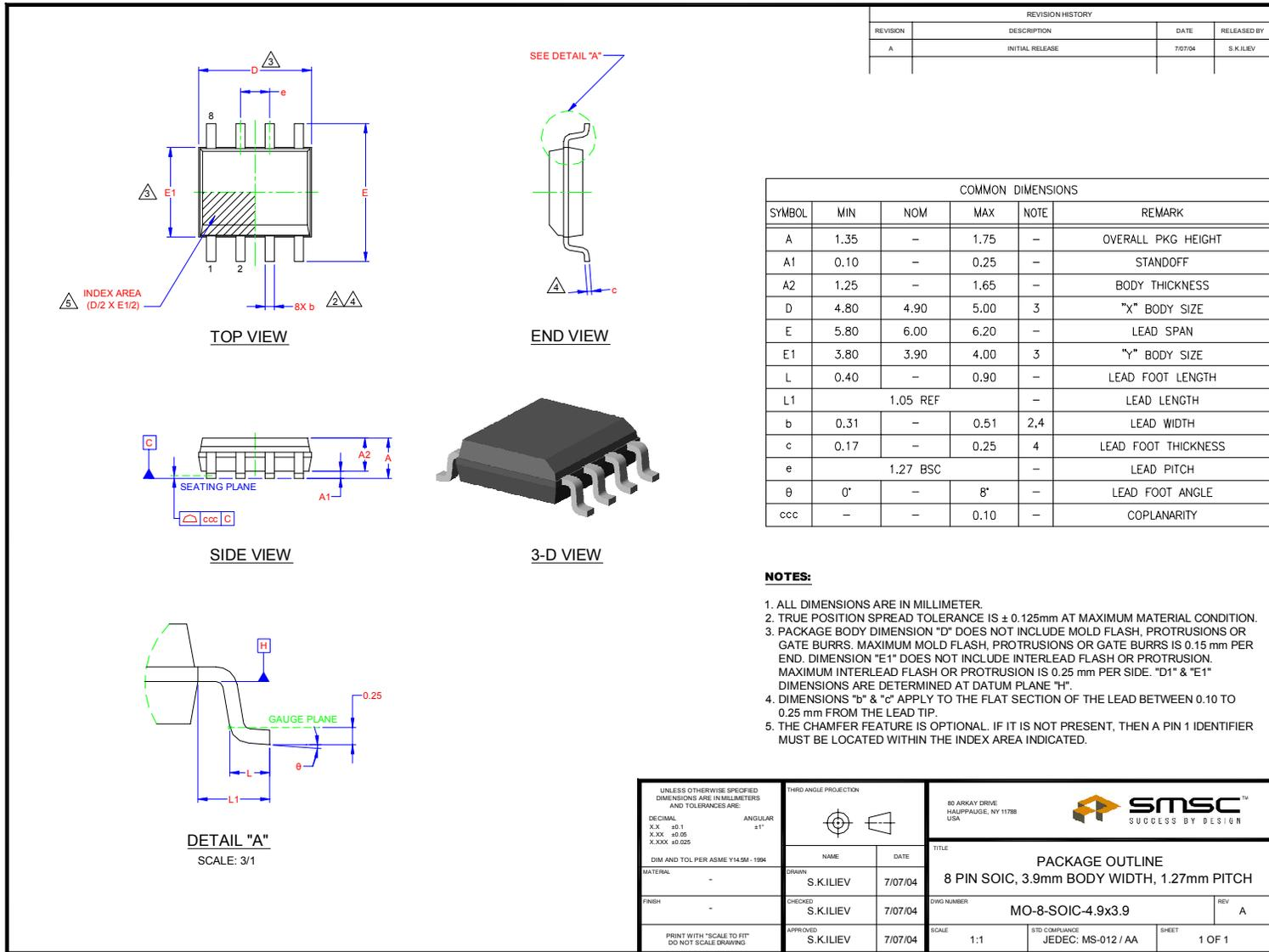
Figure 2 8-Pin SOIC Package Outline and Parameters - 3.9mm Body, 1.27mm Pitch
