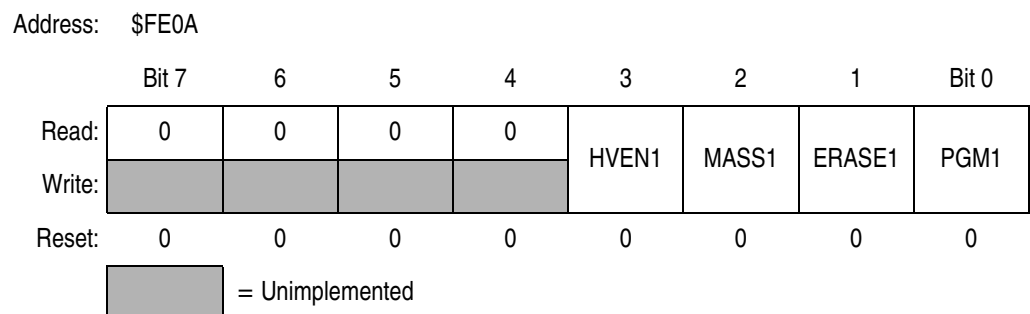
Figure 4-3. 13K-byte FLASH Control Register (FLCR1)
