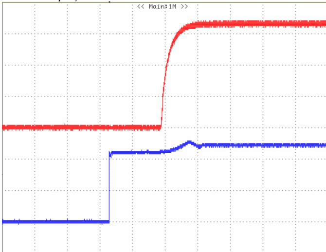
Figure 6: Turn-on transient at full rated load current (CC mode) (5ms/div). V_{in}=48V . Top Trace: V_{out} , 2V/div; Bottom Trace: input voltage, 20V/div
