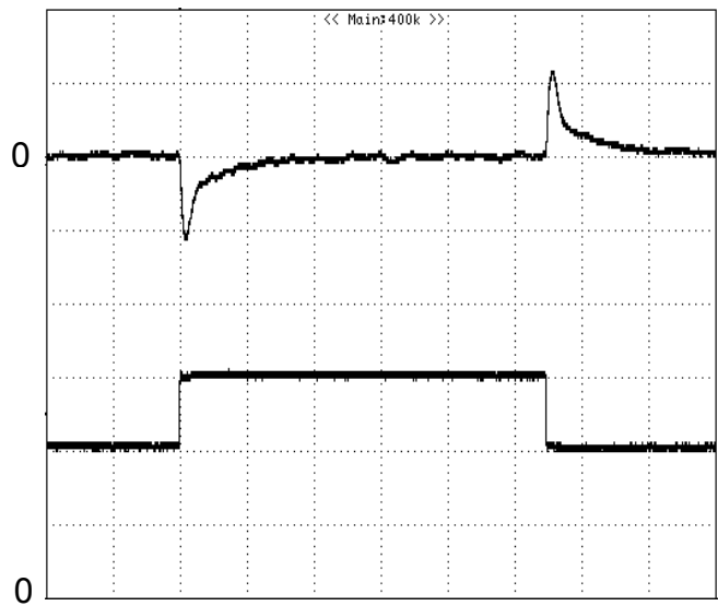
Figure 9: Output voltage response to step-change in load current (75%-50%-75% of I_o , max; di/dt = 2.5A/\mu s ). Load cap: 470\mu F , 35m\Omega ESR solid electrolytic capacitor and 1\mu F ceramic capacitor. Top Trace: V_{out} (50mV/div, 200us/div), Bottom Trace: I_{out} (5A/div). Scope measurement should be made using a BNC cable (length shorter than 20 inches). Position the load between 51 mm to 76 mm (2 inches to 3 inches) from the module
