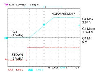
Figure 13. Shutdown/Power-Up (V<sub>in</sub> = V<sub>out</sub> + 0.5 V, I<sub>load</sub> = 50 mA)
