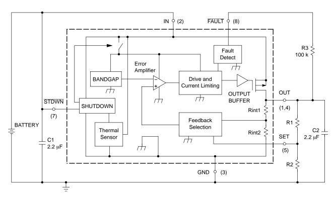
Figure 15. With External Output Voltage Adjustment
