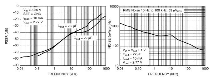
Figure 7. Power Supply Rejection Ratio
