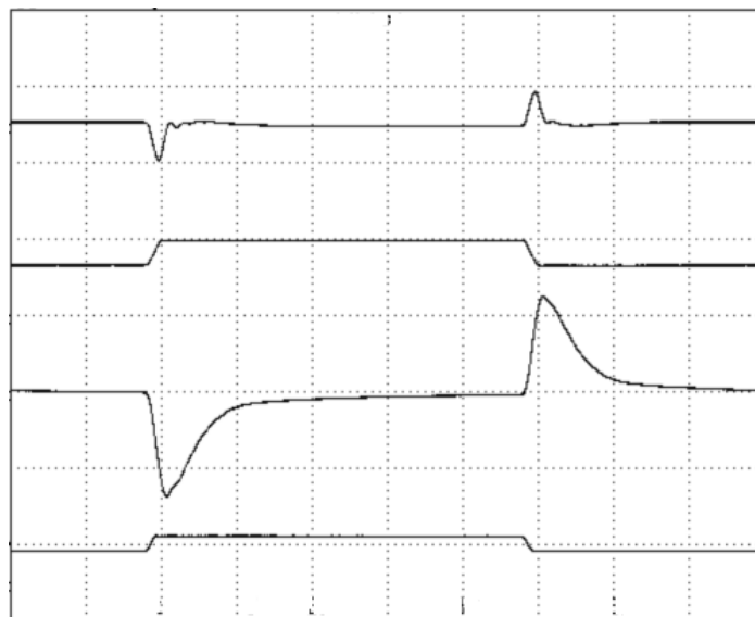
Figure 12: Output voltage response to step-change in load current I_{out2} and I_{out1} (75%-50%-75% of I_o , max; di/dt = 0.1A/\mu s ). Load cap: 10\mu F , tantalum capacitor and 1\mu F ceramic capacitor. Ch1= V_{out1} (50mV/div), Ch2= I_{out1} (10A/div), Ch3= V_{out2} (100mV/div), Ch4= I_{out2} (10A/div) Scope measurement should be made using a BNC cable (length shorter than 20 inches). Position the load between 51 mm to 76 mm (2 inches to 3 inches) from the module.
