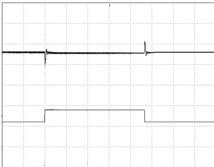
Figure 14: Output voltage response to step-change in load current I_{out1} (75%-50%-75% of I_o , max; di/dt = 2.5A/\mu s ) at I_{out2}=0A , Load cap: 470\mu F , 35m\Omega ESR solid electrolytic capacitor and 1\mu F ceramic capacitor. Ch1=V_{out1} (50mV/div), Ch2=I_{out1} (5A/div), Scope measurement should be made using a BNC cable (length shorter than 20 inches). Position the load between 51 mm to 76 mm (2 inches to 3 inches) from the module.
