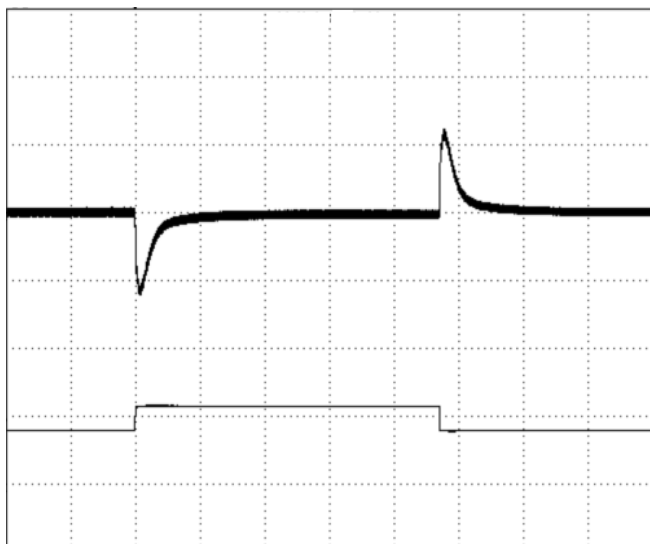
Figure 13: Output voltage response to step-change in load current I_{out2} (75%-50%-75% of I_o , max; di/dt = 2.5A/\mu s ) at I_{out1}=0 . Load cap: 470\mu F , 35m\Omega ESR solid electrolytic capacitor and 1\mu F ceramic capacitor. Ch1=V_{out2} (50mV/div), Ch2=I_{out2} (5A/div), Scope measurement should be made using a BNC cable (length shorter than 20 inches). Position the load between 51 mm to 76 mm (2 inches to 3 inches) from the module.
