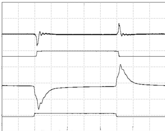
Figure 15: Output voltage response to step-change in load current I_{out2} and I_{out1} (75%-50%-75% of I_o , max; di/dt = 2.5A/\mu s ). Load cap: 470\mu F , 35m\Omega ESR solid electrolytic capacitor and 1\mu F ceramic capacitor. Ch1=V_{out1} (50mV/div), Ch2=I_{out1} (10A/div), Ch3=V_{out2} (100mV/div), Ch4=I_{out2} (10A/div) Scope measurement should be made using a BNC cable (length shorter than 20 inches). Position the load between 51 mm to 76 mm (2 inches to 3 inches) from the module.
