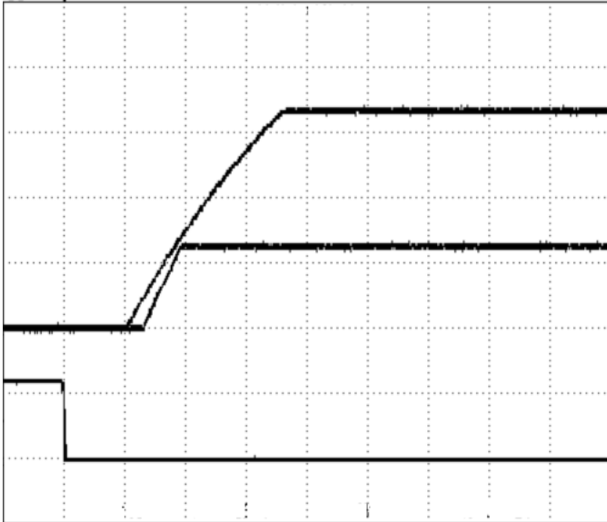
Figure 5: Turn-on transient at zero load current (5ms/div). V_{in}=48V . Negative logic turn on. Top Trace: V_{out} ; 1V/div; Bottom Trace: ON/OFF input: 5V/div
