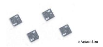
Thin film resistors are often an excellent solution for analog design problems where space is limited and high packing density is required. Due to their Tantalum Nitride resistive layer these resistors are stable 0.07 % (2000 hours, rated power at 70 °C) and moisture resistant.
