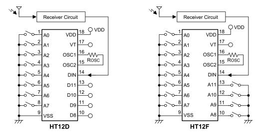
Notes: Typical infrared receiver: PIC-12043T/PIC-12043S (KODESHI CORP.) or LTM9052 (LITEON CORP.)
