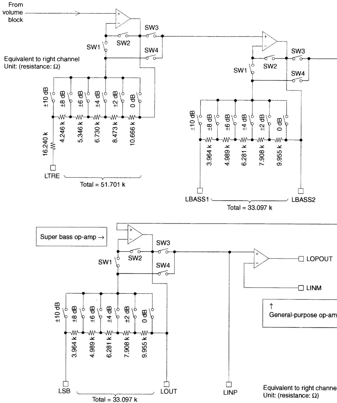
During boost, SW1 and SW3 are on, during cut, SW2 and SW4 are on, when 0 dB, 0dB SW and SW2 and SW3 are on.
