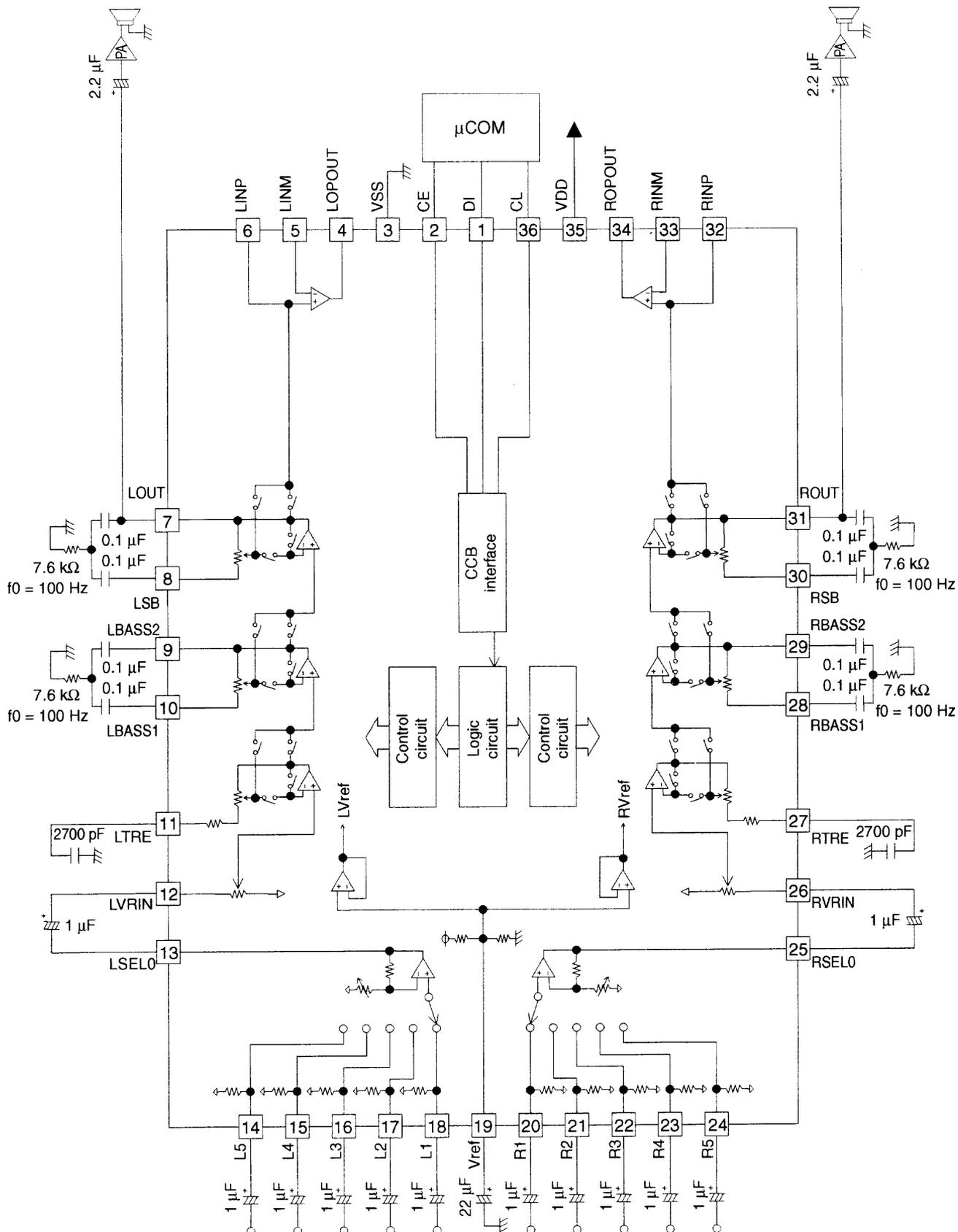
Note: When a general-purpose amp is not used, leave the LINP (RINP) open and connect the LINM (RINM) with the LOPOUT (ROPOUT).
