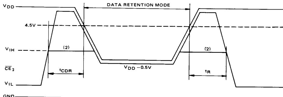
Note: (2) If the  $V_{IH}$  level of  $\overline{CE}_2$  is 2.2V, during the period that the  $V_{DD}$  voltage is going down from 4.5V to 2.7V,  $I_{SSD1}$  current flows. (Refer to D.C. CHARACTERISTICS or TYPICAL CHARACTERISTIC FIGURES.)
