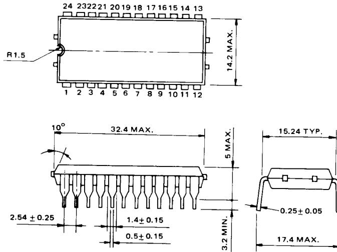
Note : Each lead pitch is 2.54mm. All leads are located within 0.25mm of their true longitudinal position with respect to No. 1 and No. 24 leads.
