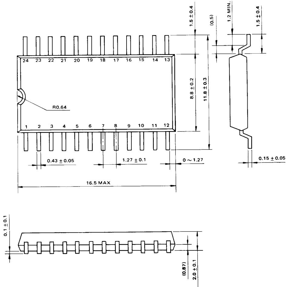
Note : Each lead pitch is 1.27mm. All leads are located within 0.1mm of their true longitudinal position with respect to No.1 and No.24 leads.
