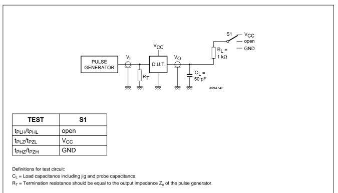
Fig.6 Load circuitry for switching times.
