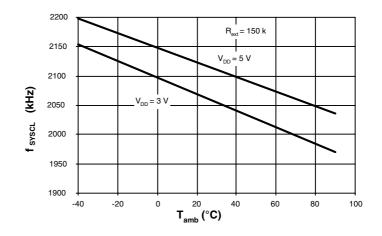
Figure 7-6.  $f_{SYSCL} = f(R_{ext})$
