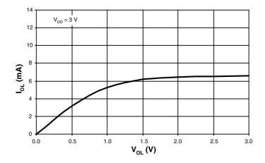
**Figure 7-13.** Typical Low Output Driver,  $V_{DD} = 5 \text{ V}$
