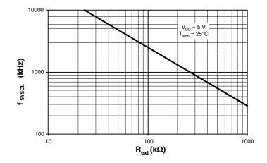
Figure 7-7.  $f_{SYSCL} = f(V_{DD}, R_{ext})$
