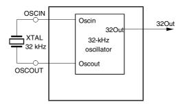
Note: Both, the 4-MHz and the 32-kHz crystal oscillator, use an integrated 14 stage divider circuit to stabilize oscillation before the oscillator output is used as system clock. This results in an additional delay of about 4 ms for the 4-MHz crystal and about 500 ms for the 32-kHz crystal.
