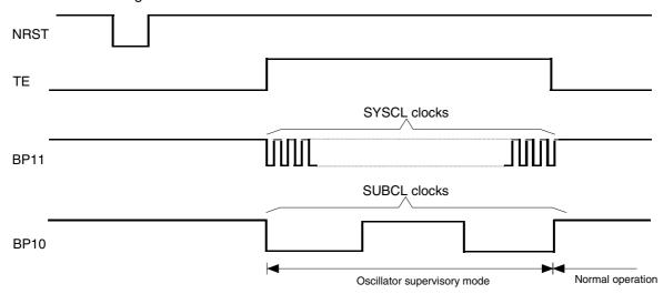
For trimming purposes, the ATAM510 can be put into a clock monitor mode. By forcing the test input (TE) high, the SYSCL clock will appear on BP11 (Port 1, bit 1) and SUBCL clock on Port BP10 (Port 1, bit 0). On releasing the TE pin, the BP10 and BP11 will resume their normal function (see Figure 2-15).
