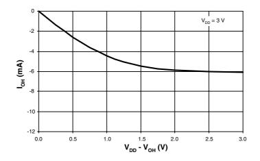
**Figure 7-12.** Typical Low Output Driver,  $V_{DD} = 3 \text{ V}$
