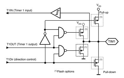
TIM1 is a dedicated bi-directional I/O stage for signal communication to and from Timer 1 in the timer/counter module (see Figure 3-8). It has no I/O bus interface and is not directly accessible from the CPU. Direction control is performed from the timer/counter configuration registers.
