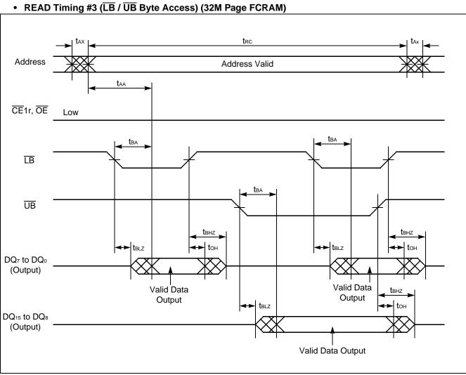
Note : CE2r and  $\overline{\text{WE}}$  must be High for entire read cycle.
