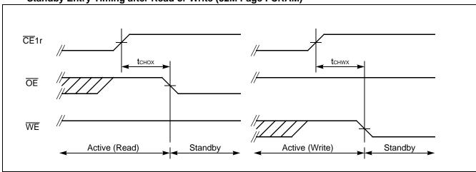
Note: Both tchox and tchwx define the earliest entry timing for Standby mode. If either of timing is not satisfied, it takes trc (Min) period for Standby mode from  $\overline{CE}1r$  Low to High transition.
