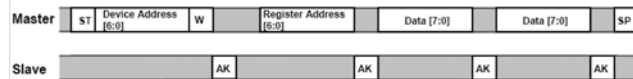
Figure 10. Multiple Byte Writes - The Master (MCU) is writing to multiple sequential registers of the MMA7450L
