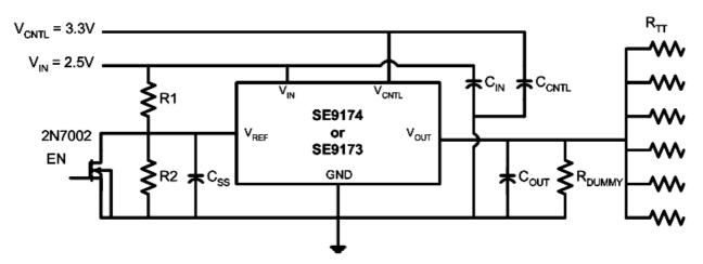
$R_1 = R_2 = 100 \text{K}\Omega$ ,  $R_{TT} = 50\Omega/33\Omega/25\Omega$
