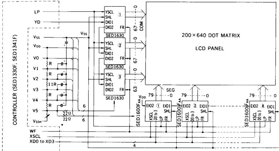
\* Be sure to connect a current limiter resistor. Also, connect decoupling capacitors (0.01 $\mu$ F) near pins Vss and V5 of each LSI for noise protection.
