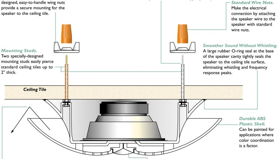
Wide Dispersion of Sound. A combination of direct and reflected sound paths produce a clear, wide dispersion of high-quality sound, even at higher frequencies where other speakers begin to beam. This enhances intelligibility and makes exact speaker placement less critical.
