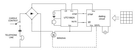
Fig.16 Typical applications of the UTC1062A (simplified)
