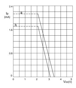
(a) Ip=2.1mA (b) Ip=1.7mA Iline=15mA at VLN=4V R1=620 $\Omega$  and R9=20 $\Omega$
