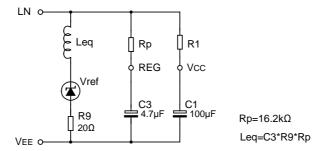
Fig.3 Equivalent impedance circuit
