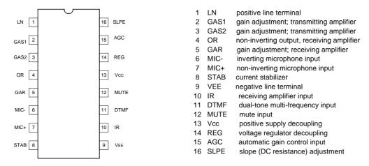
Fig.2 Pining Diagram
