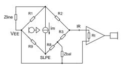
Fig 4 Equivalent circuit of UTC1062A anti-sidetone bridge
