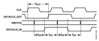
Figure 3. Double Datarate (DDR) Mode
