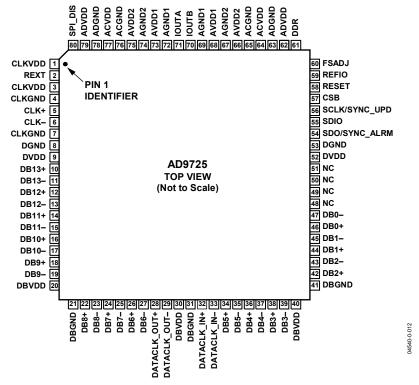
Figure 4. Pin Configuration
