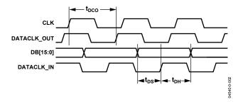
Figure 2. Single Datarate (SDR) Mode
