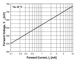
Figure 6. Forward Voltage vs
