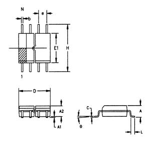
The chamfer on the body is optional. If it is not present, a terminal 1 identifier must be positioned so that one-half or more of its area is contained in the hatched zone.
