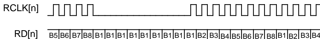
Fig. 14 Unchannelized Transmit Link Timing With Byte Synchronization
