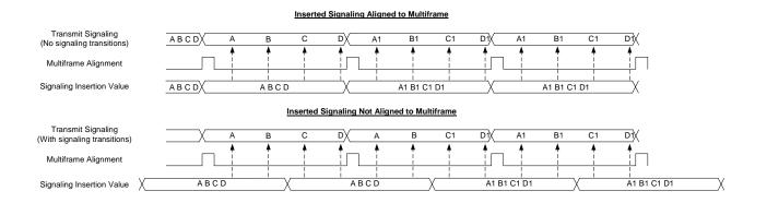
When the transmit backplane is configured for basic frame mode, the COMET assumes an arbitrary multiframe alignment. When configured for basic frame alignment, there is no way to align to the internal multiframe. Therefore transitional states for signaling might occur. Hence, it is necessary to configure the backplane for multiframe alignment to ensure signaling insertion occurs without transitional states.
