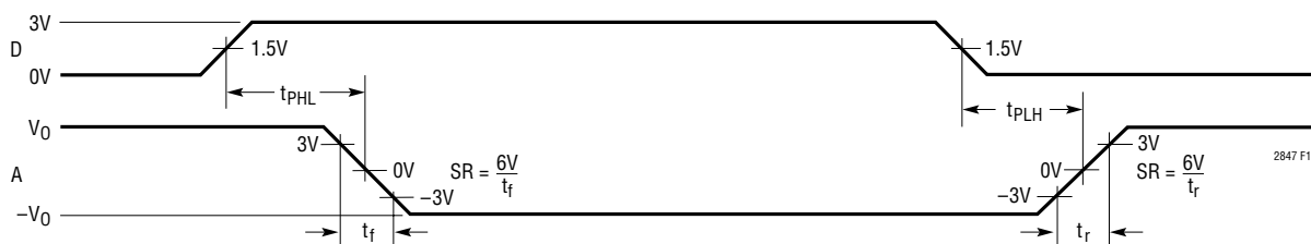
Figure 15. V.28 Driver Propagation Delays
