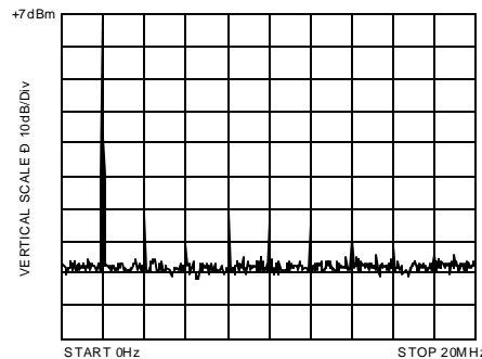
Figure 108. THD of Low Distortion Line Driver at 2 MHz
