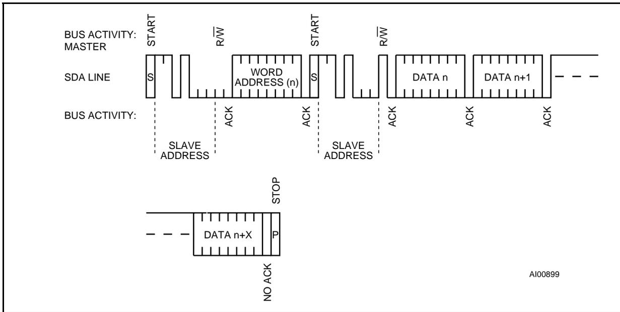
Figure 12. Alternate Read Mode Sequence
