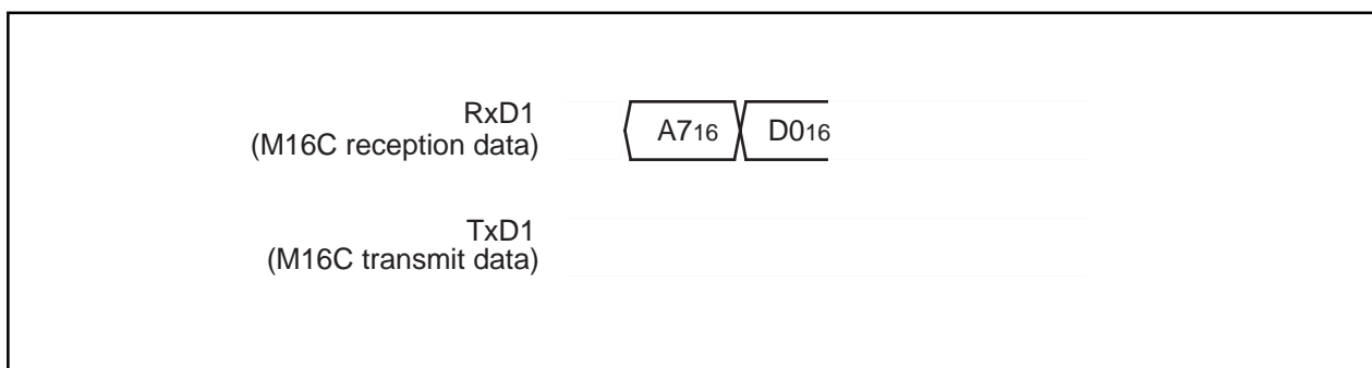
Figure 1.32.27. Timing for erasing all unlocked blocks
