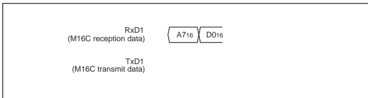
Figure 1.32.28. Timing for erasing all unlocked blocks
