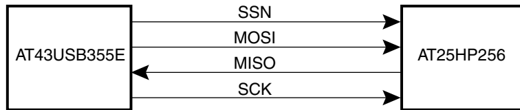
Figure 4. AT43USB355E Read Sequence
