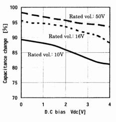
Fig.26 Capacitance change-Bias characteristic (B type) (Reference)
