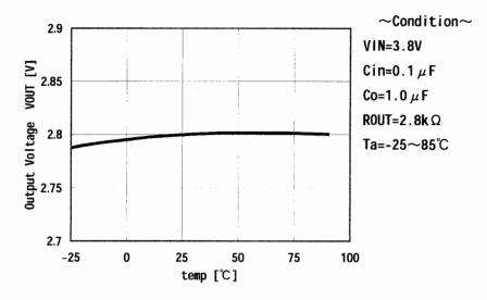
Fig.21 Output Voltage- Temperature
