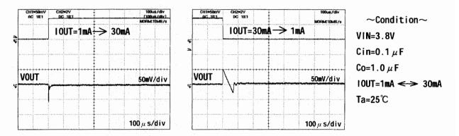
Fig.15 Load Transient response (Co=1.0  $\mu$ F)
