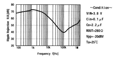
Fig. 18 Ripple Rejection - Frequency
