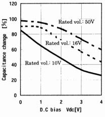
Fig.25 Capacitance change-Bias characteristic (F type) (Reference)
