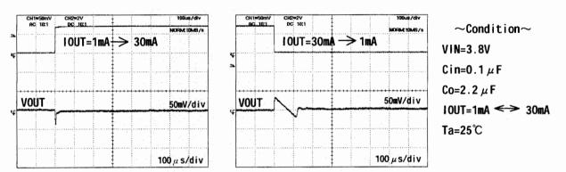
Fig. 16 Load Transient response (Co=2.2  $\mu$ F)
