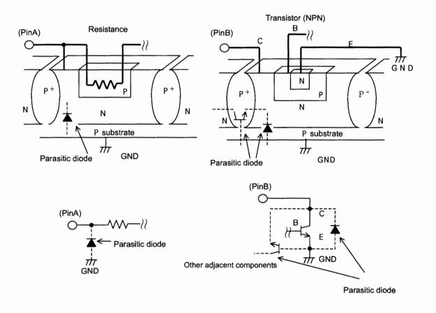
Fig.28 Simplified structure of a Monolithic IC
