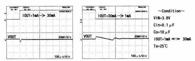
Fig. 17 Load Transient response (Co=10  $\mu$ F)
