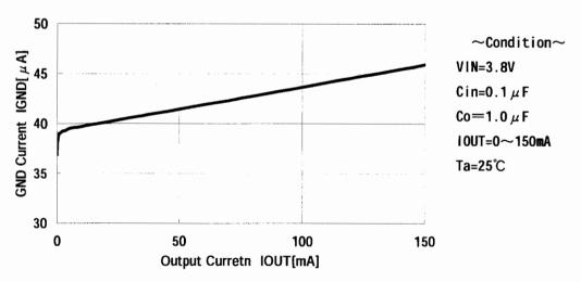
Fig. 12 GND Current-Output Current
