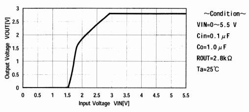
Fig.10 Output Voltage-Input Voltage
