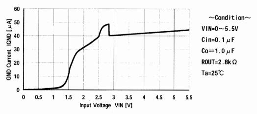
Fig.11 GND Current-Input Voltage
