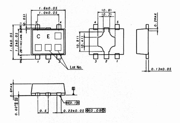
Fig.1 PACKEGE (Plastic Mold) (Unit:mm)
