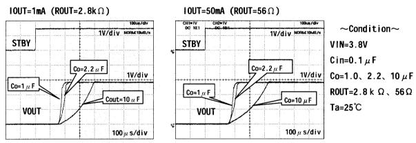
Fig.19 Output Voltage Start-up time
