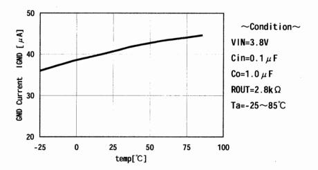
Fig. 22 GND Current- Temperature
