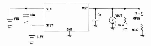
Fig.5 Load excessive response (Characteristic example: Fig.15~17)
