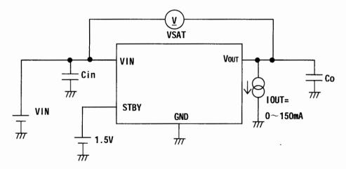
Fig.8 Input.output voltage difference Test Circuit (Characteristic example: Fig.14)
