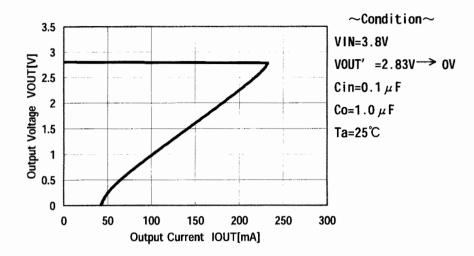
Fig.13 Output Voltage-Output Current
