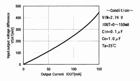
Fig.14 Input.output voltage difference—Output Current
