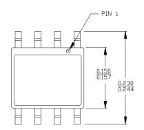
DIMENSIONS IN INCHES  $\frac{\text{MIN.}}{\text{MAX.}}$ LEAD COPLANARITY 0.004 MAX.
