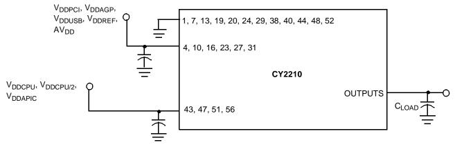
Note: Each supply pin must have an individual decoupling capacitor.
