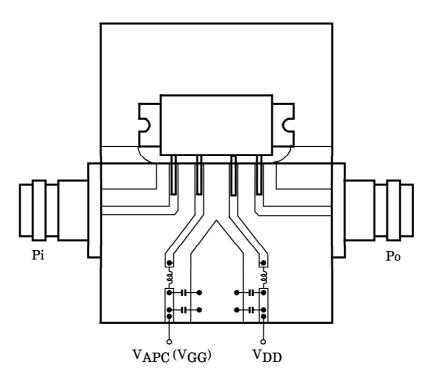
C : 10000pF,  $10\mu$ F PARALLEL L :  $\phi$ 0.5, 3ID, 5T ENAMEL WIRE
