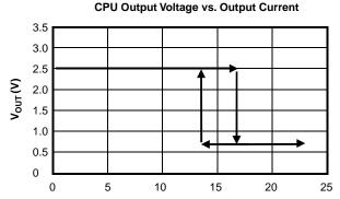
Figure 4. FAN5059 Short Circuit Characteristic
