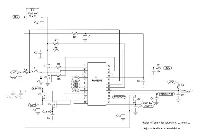
Figure 2. Application Circuit for Coppermine/Camino Motherboards (Typical Design)
